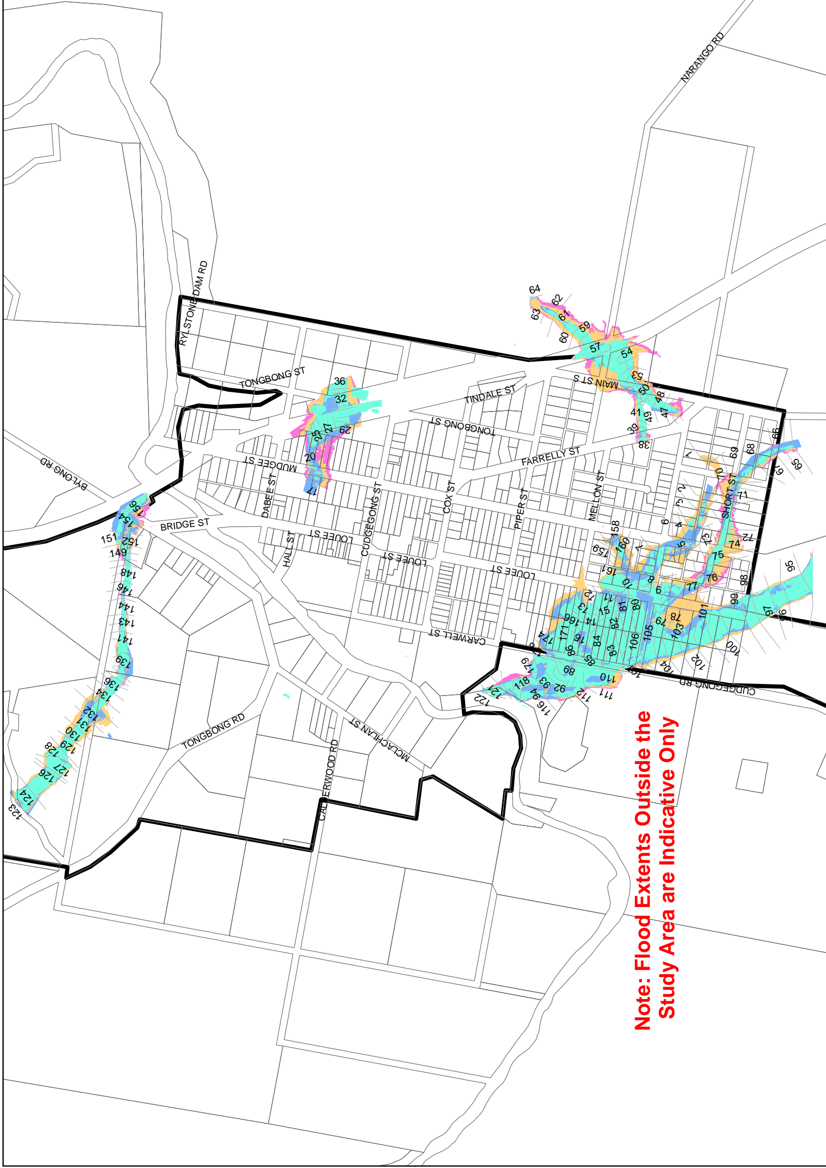
Figure 5-1 Extent of Flood Inundation in Rylstone due to Rainfall Runoff Generated from Local Catchments
