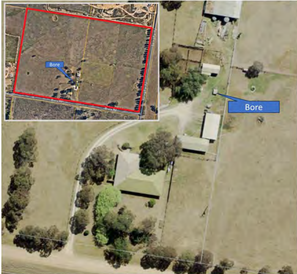
Figure 3.3: Unregistered domestic and stock water bore at the Subject Site.
