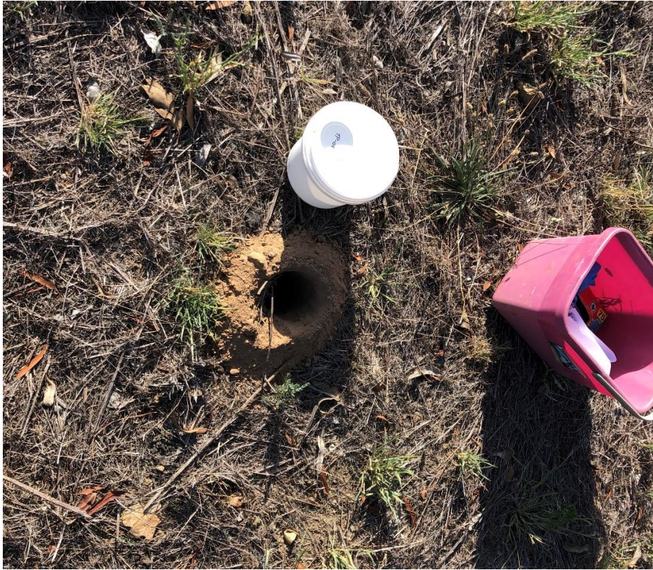
Figure 5.5: Auger hole in soft yellow sandy silt soil.
