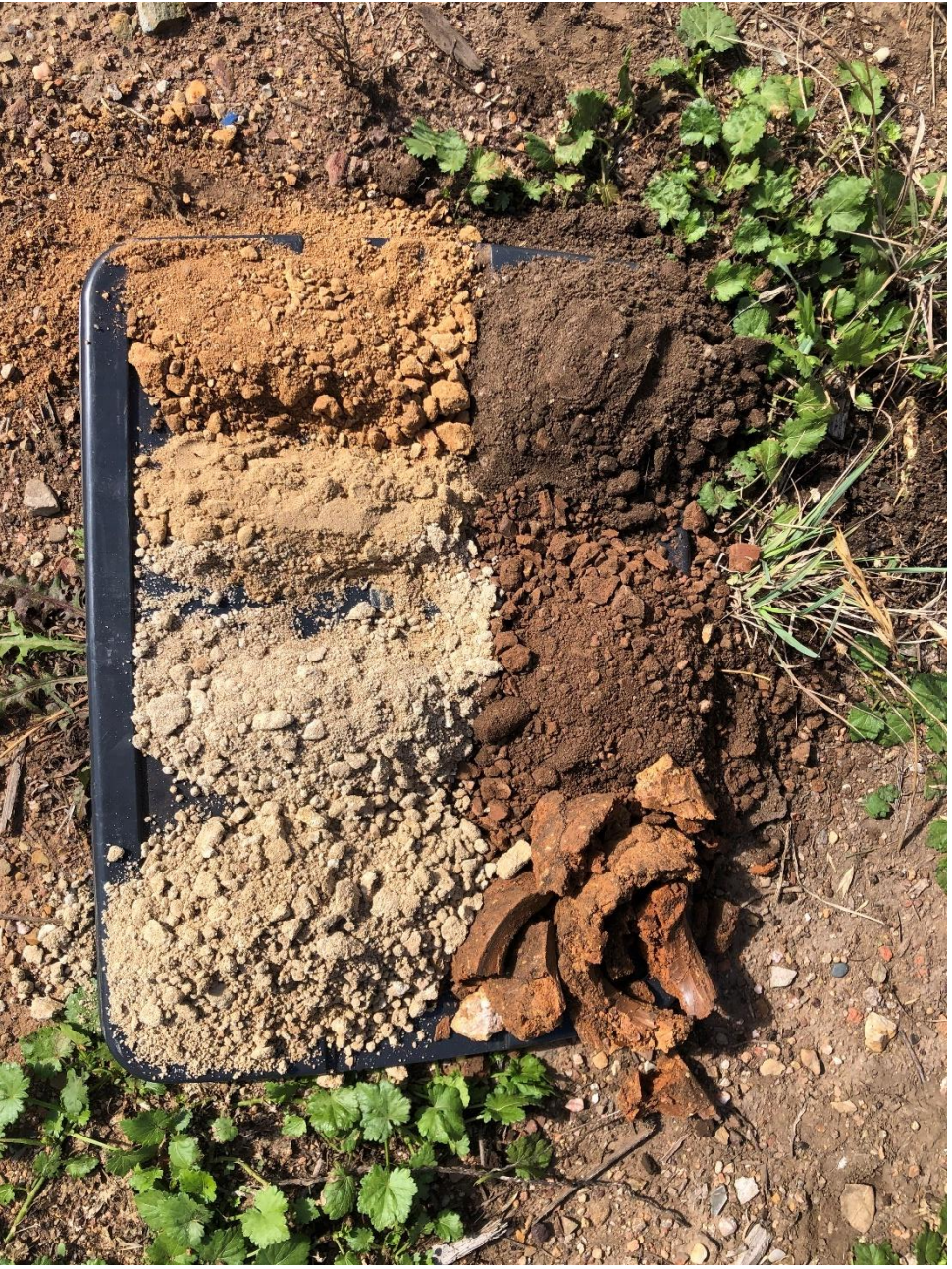
Figure 5.5: Soil samples retrieved at 500mm intervals to 3.0m from a geotechnical bore at the Subject Site.
