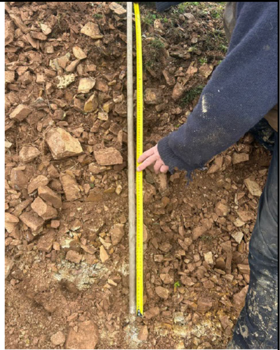
FIGURE 2.11: Test Pit 4- on eastern side of knoll, within proposed extraction area Very shallow yellow-brown sandy loam soil with rock fragments from ground level. Very gravelly/rocky.
