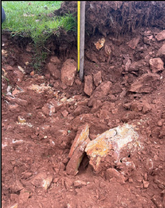
FIGURE 2.11: Test Pit 5- near top of knoll, within proposed extraction area Shallow brown loam soil with rock fragments over rock at 40-70mm. Minimal topsoil. Very rocky.
