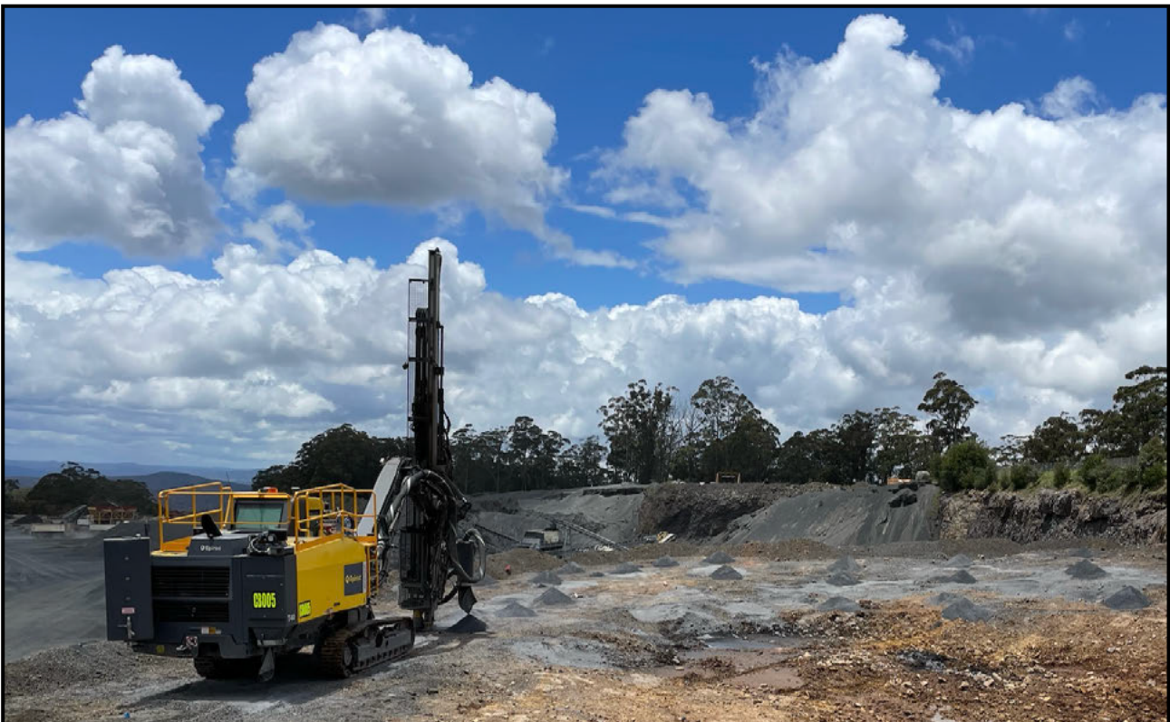
PHOTOGRAPH 3.5: Typical drill rig in the process of drilling holes for blasting at a quarry
