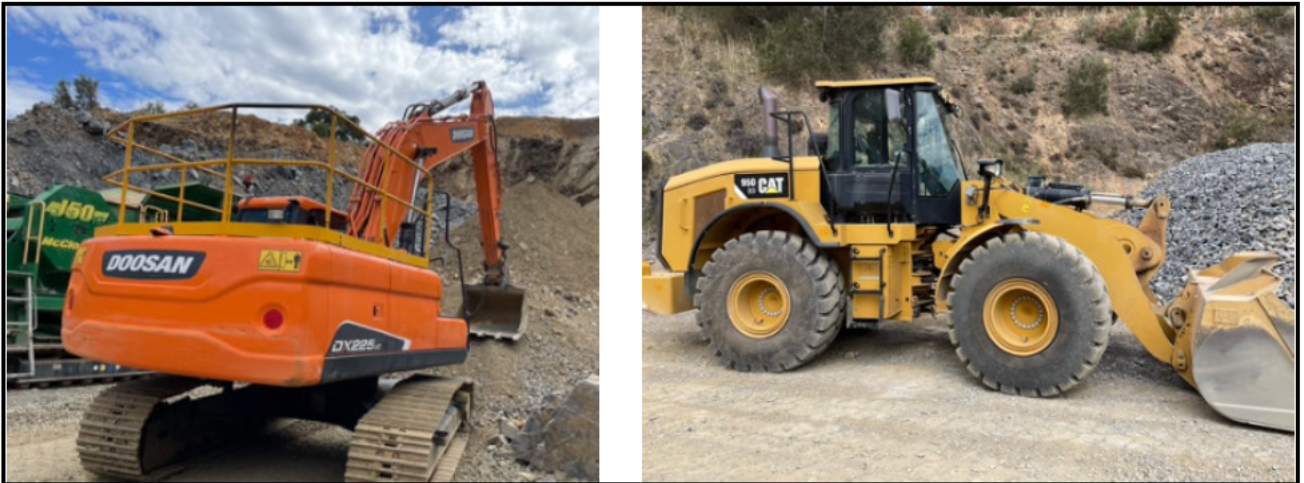
PHOTOGRAPHS 3.8 & 3.9: Typical quarry excavator (on left) and front-end loader (on right)
