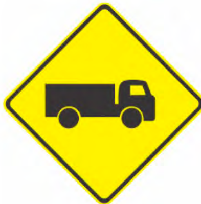
FIGURE 7.30: Typical W-22 sign face (TfNSW)
