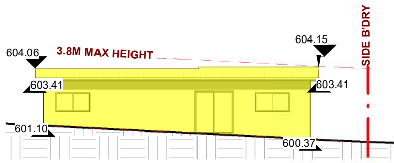
2 NOTIFIED - EAST ELEVATION 1 : 200
