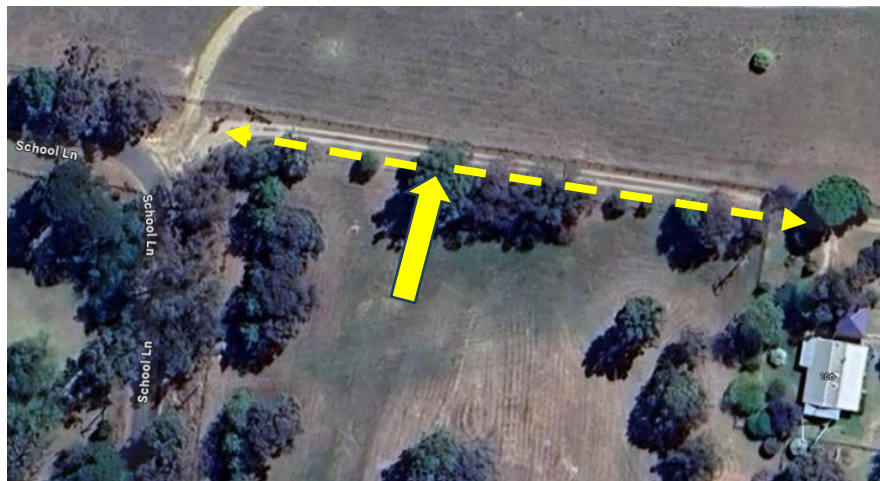
SISD distance shown at the driveway frontage
