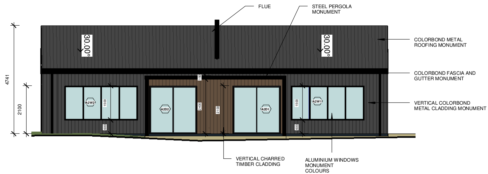
2 APARTMENT 2 - NORTH ELEVATION A301 1:100
