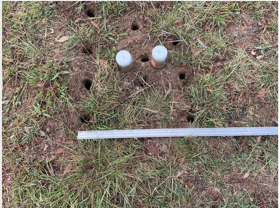
Core samples taken from 600mm x 600 mm area to fill each test site 1 through to 8
